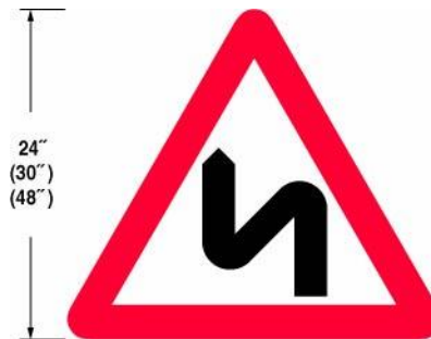
Double bend, first to the left Permitted variant: The symbol may be reversed 513
