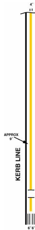
Longitudinal line to be placed on the side of a road to indicate that waiting by vehicular traffic on that side is prohibited along the length of the line (See Articles 14 and 17) 1017
