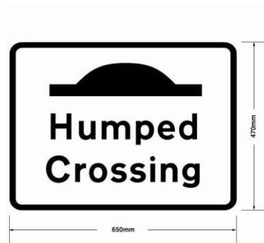
Plate for use with sign in diagram Nos. 543 or 544 in a case where a road hump is constructed and maintained in accordance with Regulation 4(4) of the Highways (Road Humps) (Jersey) Regulations 2002 547.5
