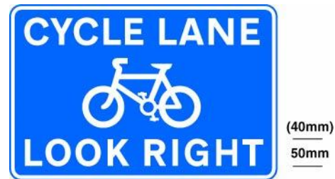
Cycle lane with traffic proceeding from right (Sign for pedestrians) Permitted variants: "RIGHT" may be varied to "LEFT" or "BOTH WAYS". "LANE" may be varied to "LANES" or "TRACK". The symbol may be reversed. 963.1
