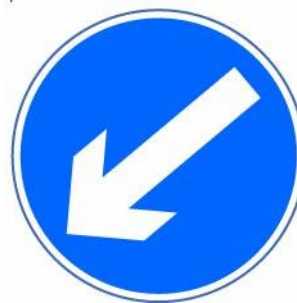
Keep left Permitted variant: The arrow may be pointed downwards to the right to indicate Keep right 610
